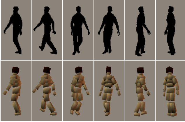
Figure 6. Some sample pose reconstructions for a spiral walking sequence not included in the training data. The reconstructions were computed with a Gaussian kernel RVM, using only 156 of the 2636 training examples. The mean angular error per d.o.f. over the whole sequence is 6.0^\circ .
