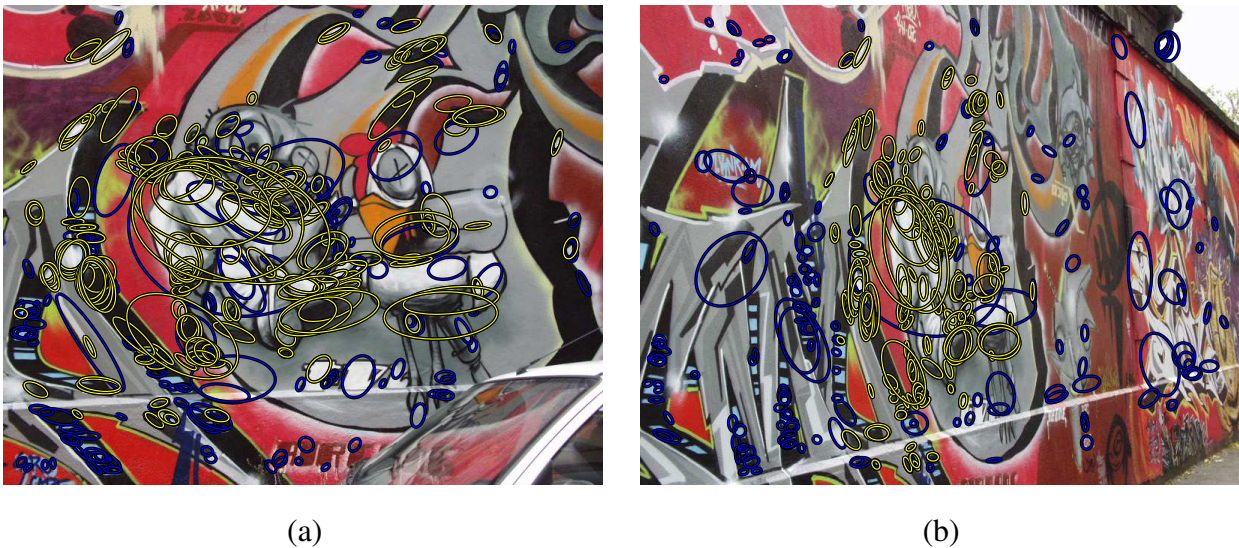
Fig. 13. Matching example. There are 400 nearest neighbor matches obtained with the GLOH descriptor on Hessian-Affine regions. There are 192 correct matches (yellow) and 208 false matches (blue).
