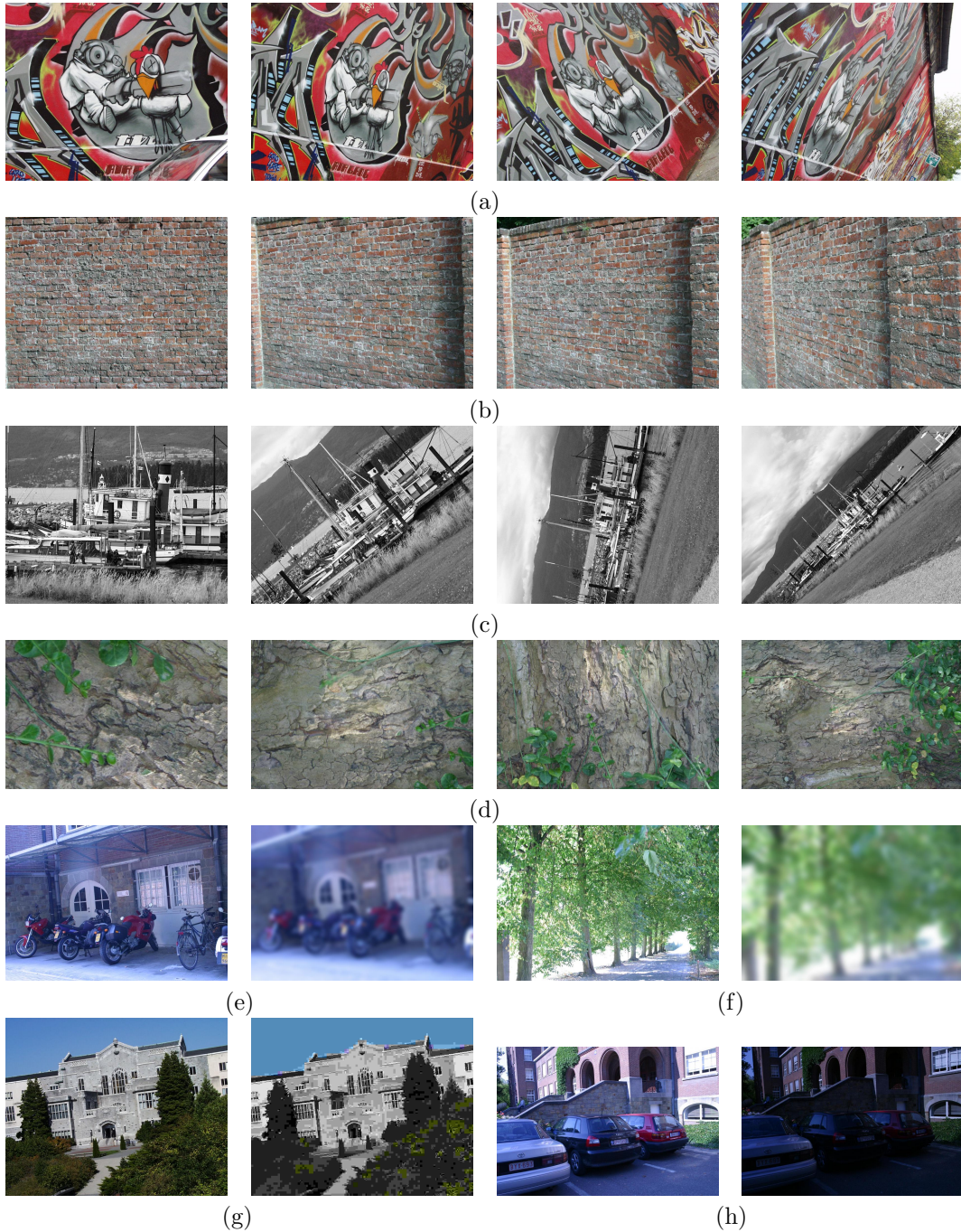
Figure 9: Data set. (a), (b) Viewpoint change, (c),(d) Zoom+rotation, (e),(f) Image blur, (g) JPEG compression, (h) Light change. In the case of viewpoint change, scale change and blur, the same change in imaging conditions is applied to two different scene types: structured and textured scenes. In the experimental comparisons, the left most image of each set is used as the reference image.
