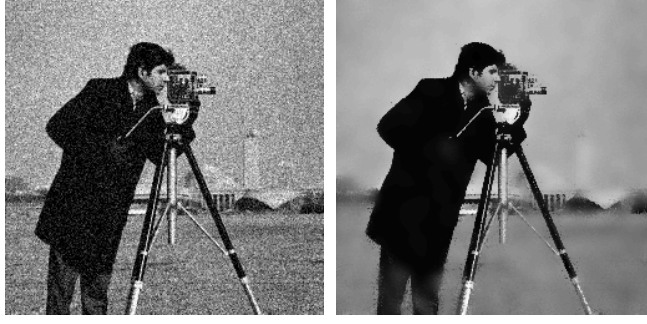
Fig. 7. Robust Estimation of Local Image Structure. On the left the camera-man image with noise added and on the right the robust estimation of the zero order coefficient in a first order facet model.
