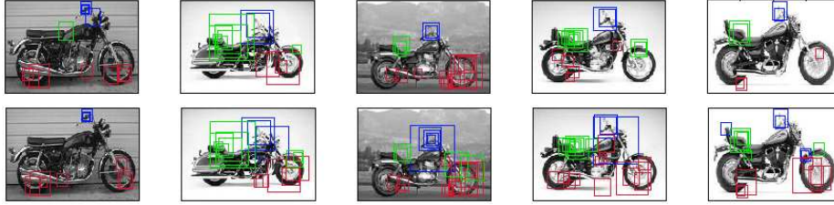
Fig. 1. Recognition of the class “motorbike” using HDDA (top) and SVM (bottom). The colors blue, red and green are respectively associated to handlebars, wheels and seat.
