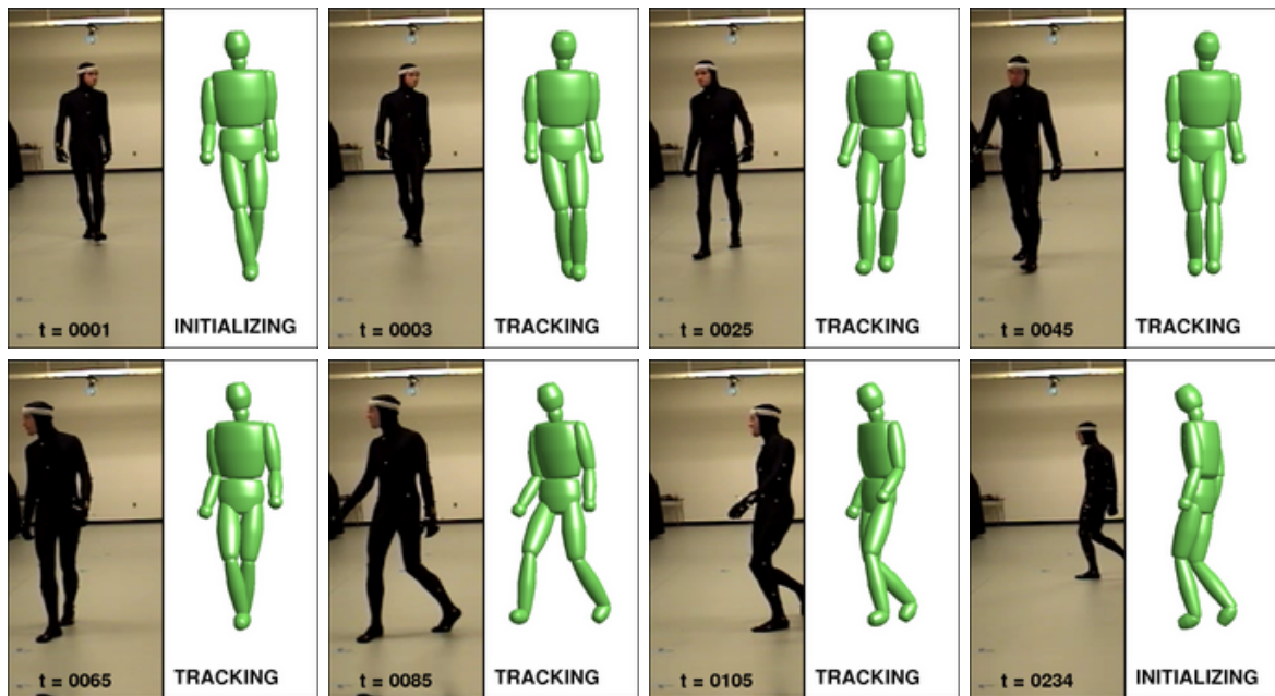
Figure 18: Multiple hypothesis tracking of a person over 500 frames using the mixture of regressors method. (Sequence taken from http://mocap.cs.cmu.edu ). Our method provides direct probabilistic pose estimation from a single image, thus allowing automatic initialization and re-initialization. Maintaining multiple track hypotheses allows the tracker to recover from possibly inaccurate initializations, tracking stably through regions in which the person is not observed.
