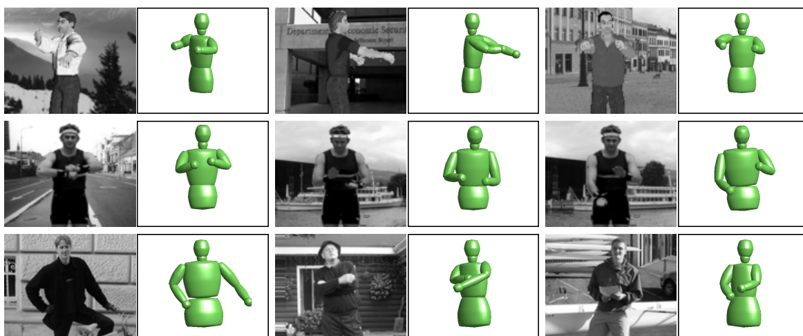
Figure 19: Pose reconstructions from our cluttered background method, on artificially rendered and real images with complex backgrounds. Top row: unseen test images with a random background image and an artificial human in a random pose synthesized using POSER. Middle row: a test sequence of a real person from our motion capture dataset, again with artificial backgrounds to make the problem more difficult. The training set included similar gestures made by another person. Bottom row: unseen real images obtained using Google. The method is purely appearance based – no segmentation of the subject is needed.
