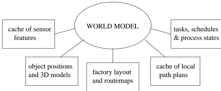
Figure 2: Types of information stored in the robot world model.
