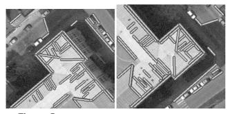
**Figure 5.** Matched line segments using the long range motion algorithm. There is a significant rotation between the images. 93% of the 55 matches shown are correct.
