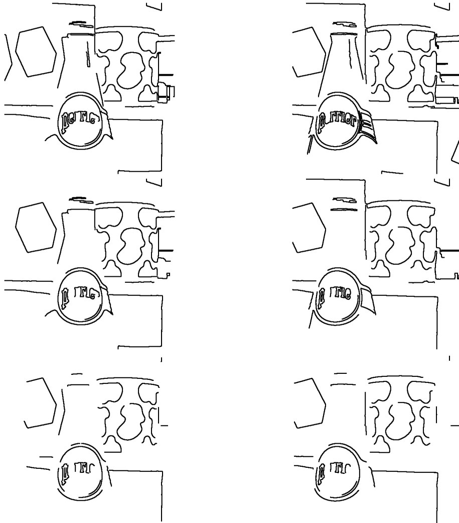
Fig. 5. Short baseline matching. Upper pair : Contours extracted with CannyOx (parameters: min grad 60, min length 60). 37 and 47 contours are obtained for the left and right images respectively; Middle pair : Contours which are matched between views. Lower pair : Matched contours showing only the parts which have corresponding edgels in both views. 97% of the 29 matches are correct.
