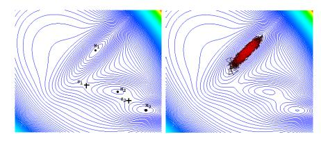
**Fig. 2.** The Müller Potential (left) and a standard stochastic dynamics gradient sampling simulation (right) that gets trapped in the basin of the starting minimum.
