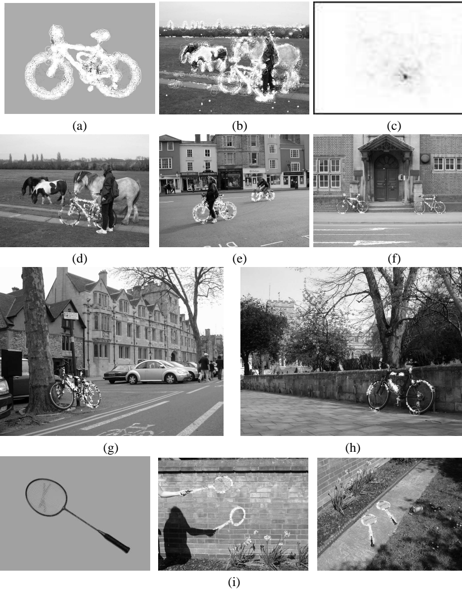
Figure 7: Examples of objects correctly recognized in images. (a) Object model, the shape is learnt from one image and the system recognizes another similar object. (b) All features detected in the target image, (c) Hyperplane of the Hough space displaying the dominant pose cluster, (d) Inliers to the estimated transformations. (e)(f) Examples with background clutter and scale changes. (g)(h) Wide viewpoint changes. (i) Another object model and matched examples.
