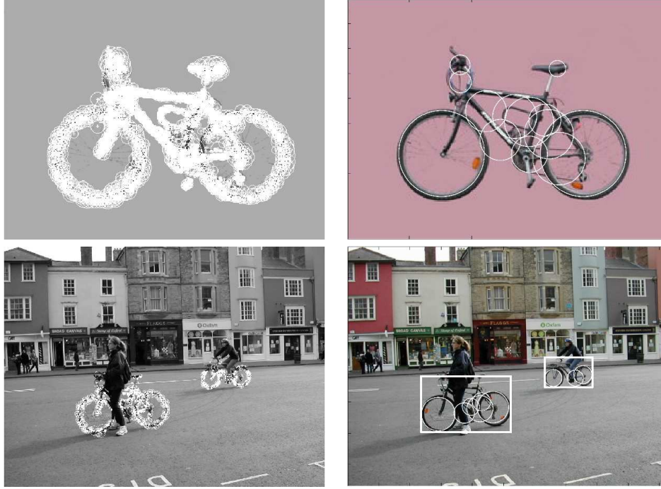
Figure 3: Detection of object categories based on shape features. Left column: edge features, right column: local shape features. Top row: features extracted for the training image, bottom row: detection results.
