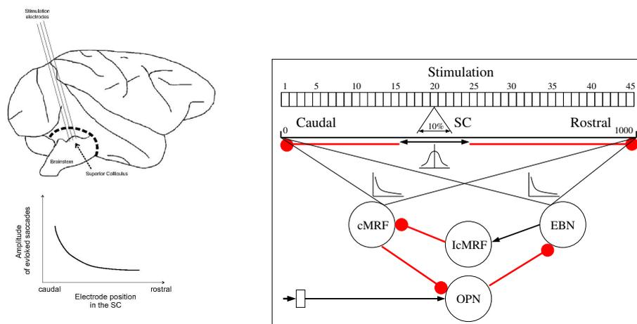
**Fig. 2.** Left : Anatomical locating of the Superior Colliculus at the top of the brainstem (top) and relationship between the amplitude of evoked saccades and the position of an electrical stimulation (bottom). Right : Topology of the modular spiking neural network. Black arrows show excitatory influence and red round ended arrows show inhibitory influence.
