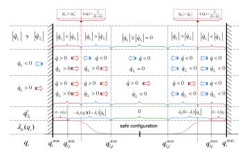
Fig. 2. Comparison between the magnitudes of the  $i^{th}$  components  $\dot{\mathbf{q}}_{\mathbf{2}}[i]$ and  $\dot{\mathbf{q}}_{\mathbf{1}}[i]$  where  $\dot{\mathbf{q}}_{i}^{i}[i]$  is defined by (17) within the different values for  $q_{i}$ of the joint  $j_{i}$  and when  $\lambda_{i} > 0$ ; Illustration of the relation between the direction of  $\dot{\mathbf{q}}_{\mathbf{1}}[i]$ ,  $\dot{\mathbf{q}}_{i}^{j}[i]$ , and  $\dot{\mathbf{q}}[i]$ .
