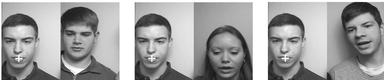
Fig. 3. Sample frames of Movie 1 [Left], Movie 2 [Center] and Movie 3 [Right]. The left person is the real speaker, the right subject mouths the same words pronounced by the speaker but his audio track has been removed. The white cross highlights the estimated position of the sound source, which is correctly placed over the speaker's mouth.
