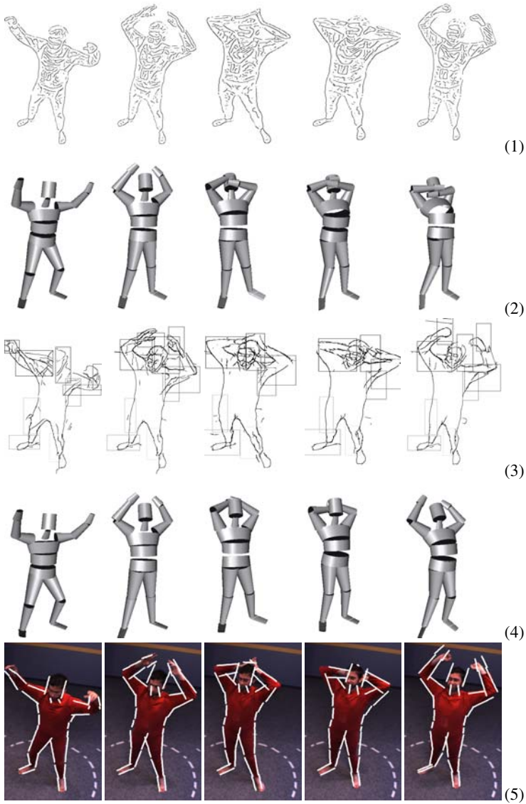
Fig. 7. Tracking of a 200-frame video sequence comparing standard edge detection method with the Anisotropic Gaussian filtering. The standard edge detection on gray level images is shown on row (1). The estimated pose is given on row (2). Note that the tracker fails: the arms are not correctly tracked. The Anisotropic Gaussian filtering (3) performs well on the arms compared to the standard method. The estimated pose is given on row (4). Last row (5) shows the extremal contours projected onto the original camera images.
