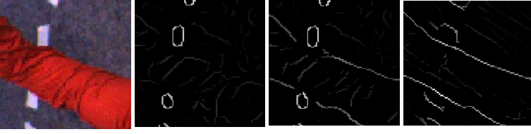
Fig. 3. (a) The arm is visible from the top view. (b) Standard Canny filter reveals markings on the ground and foldings of the clothings. (c) Color Canny filter partially detects the arm contours. (d) Anisotropic Gaussian color filter reveals the full arm contours.
