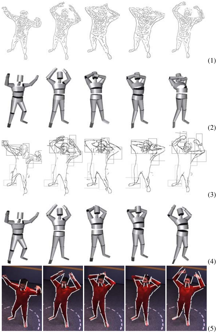
Fig. 7. Tracking of a 200-frame video sequence comparing standard edge detection method with the Anisotropic Gaussian filtering. The standard edge detection on gray level images is shown on row (1). The estimated pose is given on row (2). Note that the tracker fails: the arms are not correctly tracked. The Anisotropic Gaussian filtering (3) performs well on the arms compared to the standard method. The estimated pose is given on row (4). Last row (5) shows the extremal contours projected onto the original camera images.
