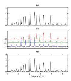
**Fig. 2.** A three note chord original spectrum (a) decomposed into (b) three weighted dictionary spectra, which combine to give the reconstruction (c).
