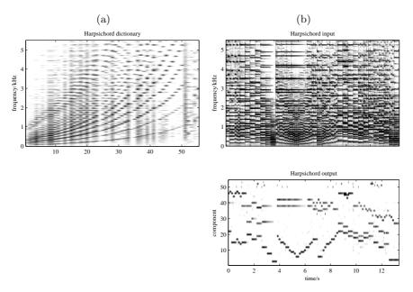
**Fig. 1.** Dictionary matrix **A** after learning (a), with (b) the original spectrum sequence  $\mathbf{x}$  (top) decomposed to the sparse representation  $\hat{\mathbf{s}}$  (bottom).
