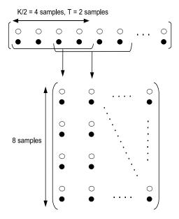
Fig. 1. Reshaping of the sensor vector prior to training with ICA. In this illustration, we have K/2=4 sample pairs per frame, with an overlap of T=2 samples. the (i,k)-th element of the new matrix,  $\bar{\mathbf{X}}$ , is given by
