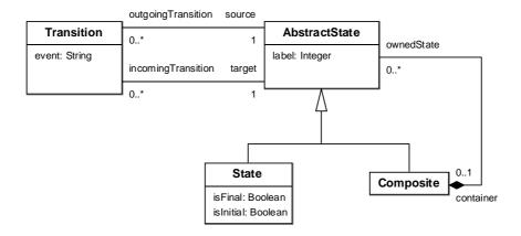
Figure 2 - A Hierarchical State Machine Metamodel.
