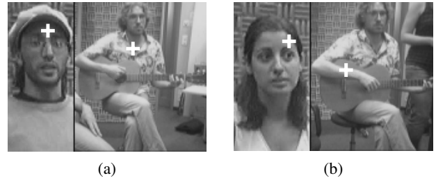
Fig. 12. Two frames belonging to movie2 (a) and movie3 (b). On both frames, one person is uttering numbers while a guitarist is playing. Frame (b) shows the distracting motion caused by a person who is crossing the scene behind the sources. The estimated source positions are marked with crosses.
