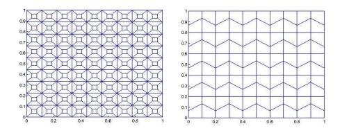
Figure 6: Meshes in honeycomb and chevron
