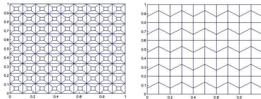
Figure 6: Meshes in honeycomb and chevron
