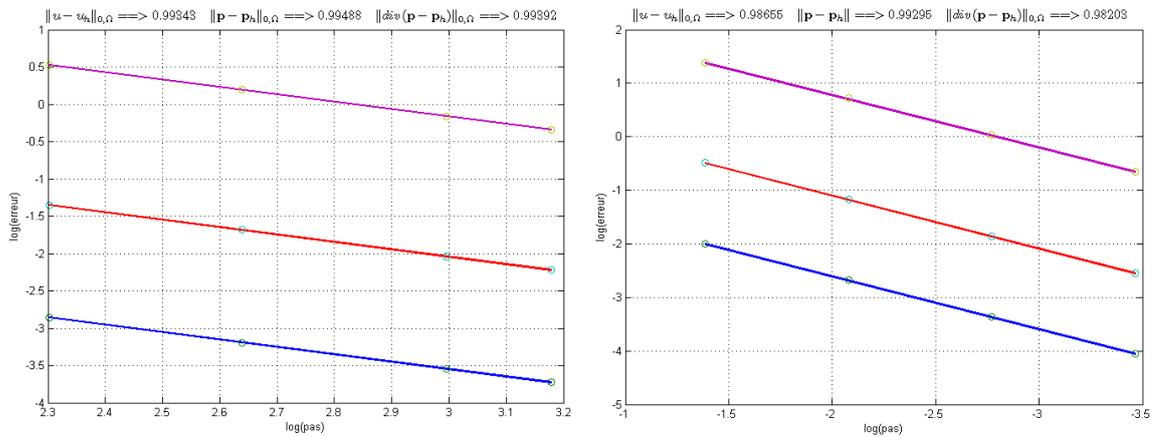
Figure 11: Convergence curves: Meshes in chevron (left), Meshes in truncated pyramid (right)
