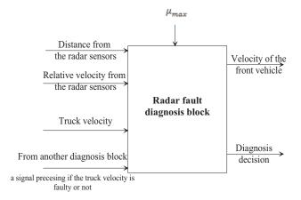
Figure 6. Radar fault diagnosis block
