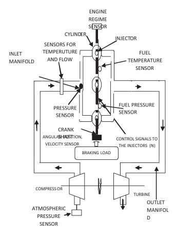
Figure 2. Engine Architecture, [10]
