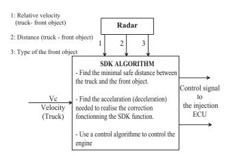
Figure 1. SDK system: algorithm and environment
