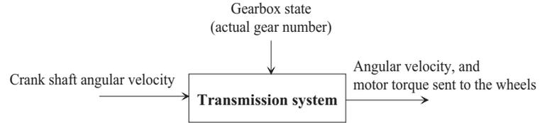
Figure 3. Transmission block
