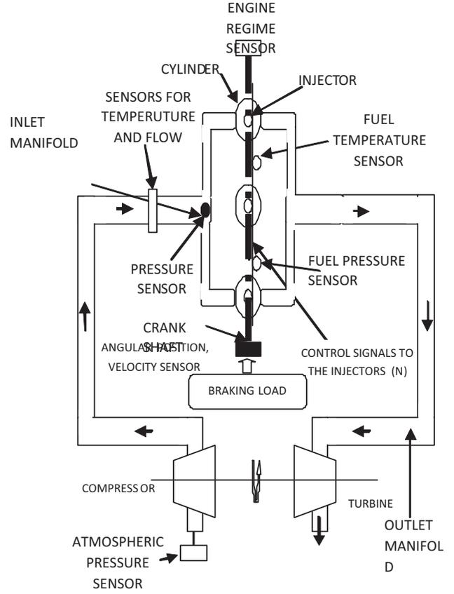
Figure 2. Engine Architecture, [10]
