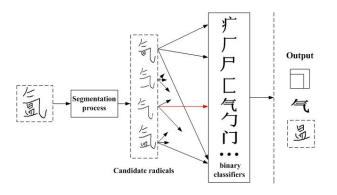
Figure 4. An example of special radical detection.
