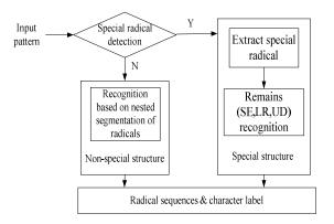
Figure 3. Framework of radical-based recognition.
