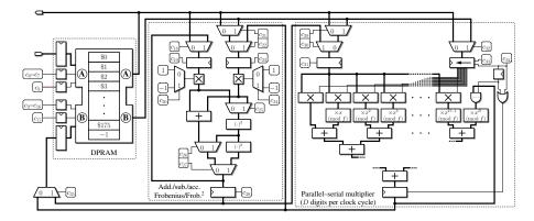
**Fig. 1.** Finite field coprocessor over  $\mathbb{F}_q$
