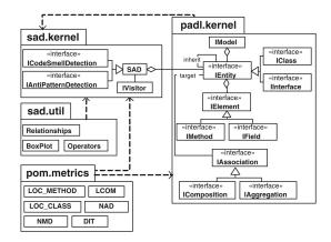
Fig. 8. Architecture of the SMELLFW framework.
