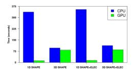
**Figure 6.** Comparison of total execution times for shape-only and shape plus electrostatic FFT calculations. Here, "CPU" refers to one core of a 3.2GHz i7-965 workstation, and "GPU" refers to a single FX-5800 GPU.
