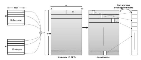
**Figure 2.** This figure illustrates a docking calculation in which multiple pairs of rotated receptor and ligand coefficient vectors are enumerated and cross-multiplied in order to calculate a series of 1D FFT correlations.
