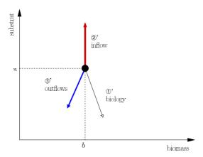
Figure 2: In this simplified model, from a position  $x = (b, s)^*$  the process could jump according to 3 mechanisms (biology, inflow, and outflow), the basic jump  $\mathfrak{G}'$  has a length  $\frac{1}{K_i'}$  for  $i = 1, \ldots, 3$
