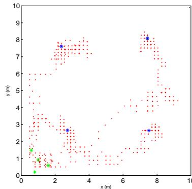
Fig. 2. Four robots with a maximum monitoring distance  $r = 3.5m$  in a convex environment. The green points show the initial positions of the robots, the final ones are in blue, in red the trajectories. The solution reproduces that one known in literature, where the robots' positions are the generator of the centroidal Voronoi partition.
