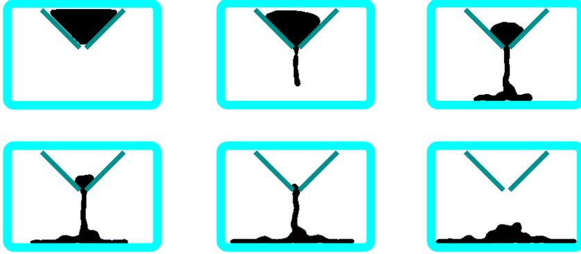
Figure 6: Snapshots from a sequence with a surface coating the particles: a quasi-liquid material (80 particles) falling under gravity.
