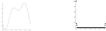
Figure 4: Left: An example of F curve, for L = (0, 1.2) , V = (1, 1.5) and \phi = .5 . It is very smooth, despite its factors are quite more chaotic. Right: the FFT of this curve. Notes that the energy is clearly concentrated on the frequencies 0, 1 and 2, thus the motivation to fit F with a linear combination of 1, \cos(\theta - \theta_A), \cos(2(\theta - \theta_B)) . NB: the values at the extreme right are the mirroring due to the FFT.
