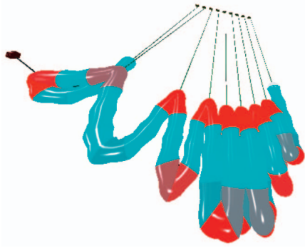
Fig. 10. Spline segment coloration to illustrate our curvature isolation process, during interactive sweep deformation.
