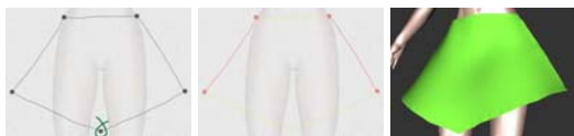
Figure 10: (left) The user has drawn a few lines to indicate the shape of the skirt; the corner-detector has detected a breakpoint that the user does not want. The user will make a deletion gesture (a curve in the shape of an \alpha enclosing the mistaken point) to delete it. (right) Here is the surface inferred by the system after the user asks for a reconstruction.
