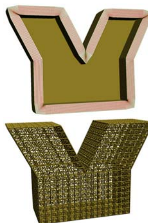
Figure 29: Left: cross-section of the shell for a shape with sharp corners; Right: same object with volume texture added.
