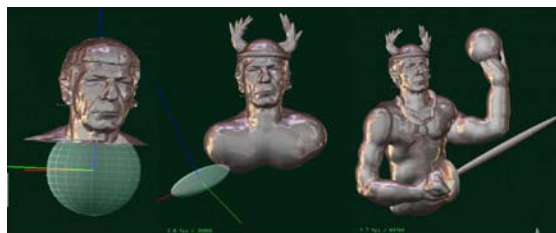
Figure 11: Three steps of a character's modelling through the editing of an imported polygonal mesh. This example illustrates multi-resolution sculpting, since large tools were used for creating a smooth body for the character while very small ones were needed to create the wings of the helmet and the chain.
