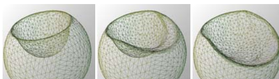
Figure 38: Behaviour of our mesh-updating algorithm on an already punched sphere. The decimation accompanying the second punch simplifies the small triangle of the first punch. The tool has been removed for better visualization.
