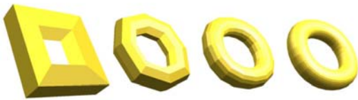
Figure 1: Subdivision defines a smooth surface recursively as the limit of a sequence of meshes.
