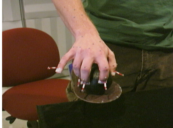
Fig. 3. Example four finger grasp collected with motion capture. Fingertips have markers on “stilts” to reduce occlusion during grasps.
