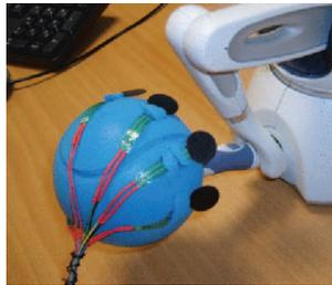
Figure 4: Foam ball with sensors
