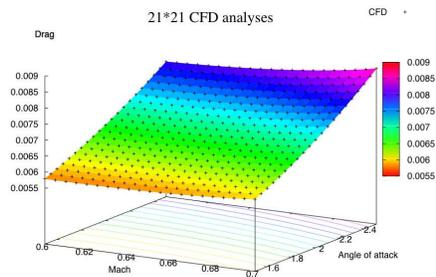
**Figure 2.** *Drag for  $21 \times 21$  CFD analyses.*
