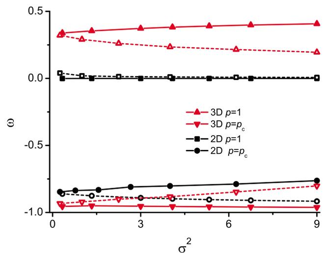
**Figure 9.** Dependence of  $\omega$  on the local permeability distribution shape for 2D square and 3D cubic networks. Solid symbols and lines stand for the log-uniform distribution while open symbols and dashed lines stand for the lognormal distribution.
