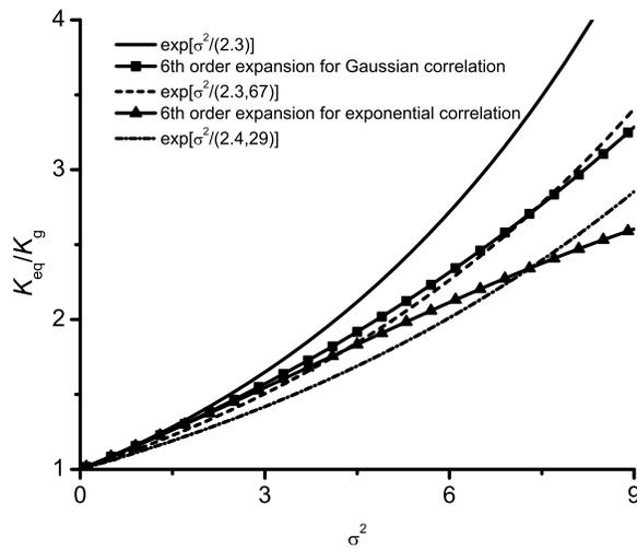
**Figure 1.** Equivalent permeability for 3D isotropic lognormal permeability fields. Plain lines with symbols indicate the 6th order approximation in  $\sigma$  [De Wit, 1995]. Fitting the sixth order expression of *de Wit* [1995] by the exponential expression (1) gives  $\omega = 1/3.67$  for the exponential case and  $\omega = 1/4.29$  for the Gaussian case. Fits are represented by the dashed and dotted curves.
