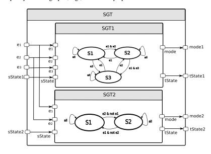
Figure 4: Parallel composition of state graph components in Gaspard.
