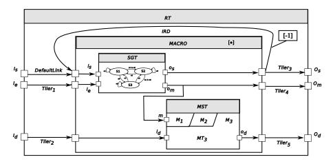
Figure 7: An example of Gaspard mode automata.
