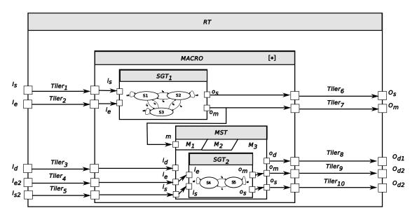
Figure 6: Hierarchical composition of state graph components in Gaspard.
