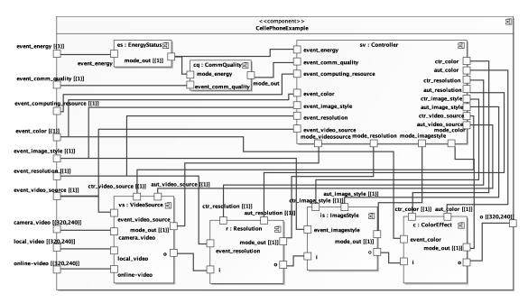
Figure 13: A global model view of the multimedia functionality module.
