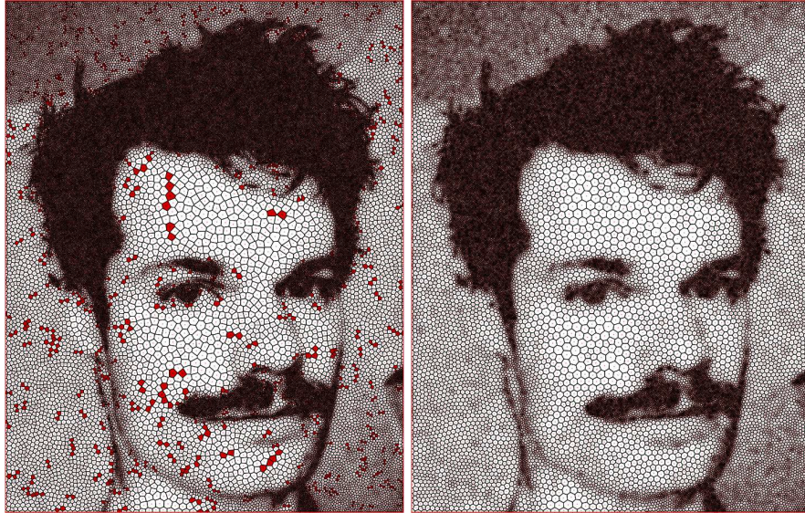
Fig. 10. CVT (left) and optimized mesh (right) for a complex highly-graded mesh generated from a photograph. The underlying Delaunay triangulation contains 113196 triangles. The condition number reduces from 354630 to 44208.
