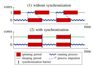
Figure 3: CPU-Hogs: using CPU burners to degrade CPU performance. Without synchronization between the spinning threads, the user process will migrate between cores and use more CPU time than allocated. This is solved in CPU-Hogs by using a synchronization barrier: there is then no advantage for the user process to migrate between cores.
