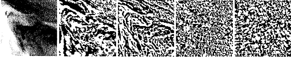
Figure 9: From left to right: spatial slice of a water vapour image at noon, t = 12 h, its temporal and spatial edges coinciding with the interfaces and regions where \sigma_{edge}^t and \sigma_{edge}^s change or have a particular sign, the ridges, ruts and inflection lines coinciding with the interfaces where \sigma_{phase} changes sign, and the ridges occur where the signature of k_i is positive. The input image acquired between t = 9 h and t = 18 h consists of 18 temporal views of spatial slices composed of 200 \times 200 voxels each with a dynamic resolution of 8 bits.
