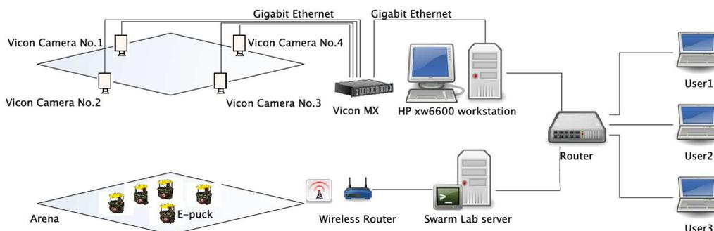
Figure 16. Experimental infrastructure for swarm robotics research based on the Linux extended e-puck. The Swarm Lab Server provides a data logging capability that combines and time stamps position tracking data collected by the Vicon™ system with robot status and sensor data from the e-pucks via WiFi, into a log file for post-analysis of experimental runs.
