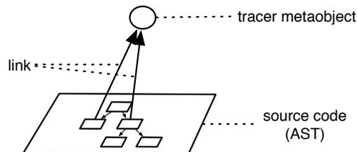
**Fig. 2.** A tracer realized with partial behavioral reflection
