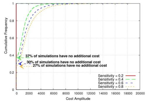
Fig. 8. Cost amplitude in function of detection sensitivity
