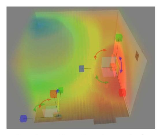
Figure 21: Temperature field estimated for a given heater position (t = 30s).
