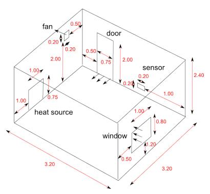
Figure 1: Configuration of the test-case.
