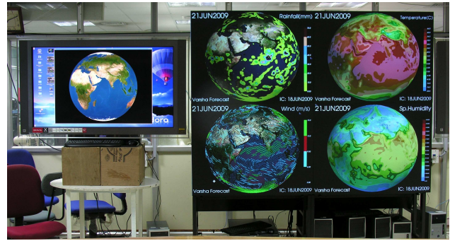
Figure 5: Four Mayavi applications controlled via the network from a central program providing a synchronized view.
