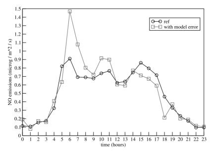
Figure 12. Optimized emissions of NO: reference values and values obtained with a model error.
