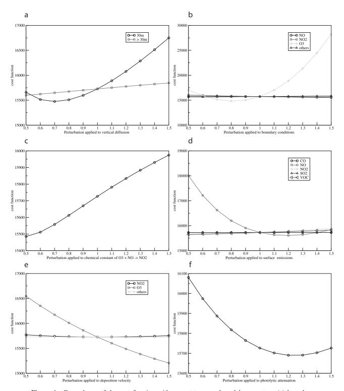
**Figure 4.** Dependence of the cost function with respect to several model parameters: (a) boundary conditions, (b)  $K_z$ , (c) kinetic rate of O3 + NO  $\rightarrow$  NO<sub>2</sub>, (d) emissions, (e) dry deposition velocities, and (f) cloud attenuation.
