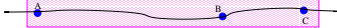
Figure 6: If a maximal blurred segment contains more than 2 dominant point candidates, the middle candidates are weak candidates of dominant point.
